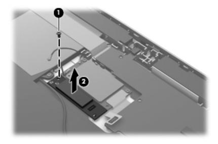
Reverse this procedure to install the GPS module.
